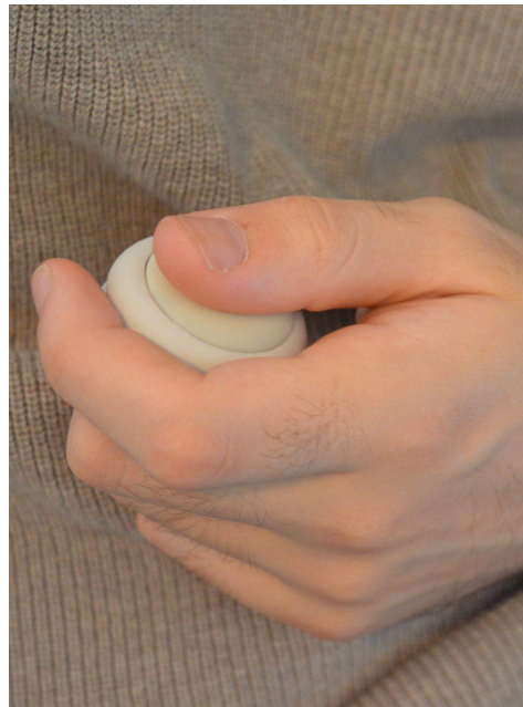
Figure 1. A photograph of the LYEONS HEART non-invasive device. The HEART provides audio and tactile heartbeat stimulus and underwent 21 days of User testing.
